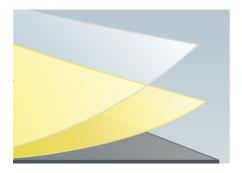
Duropal worktops are surfaced with genuine Duropal high pressure laminate produced to DIN-EN 438.
